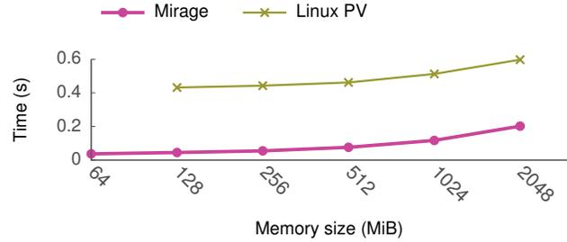
Figure 6: Boot time using an asynchronous Xen toolstack.
